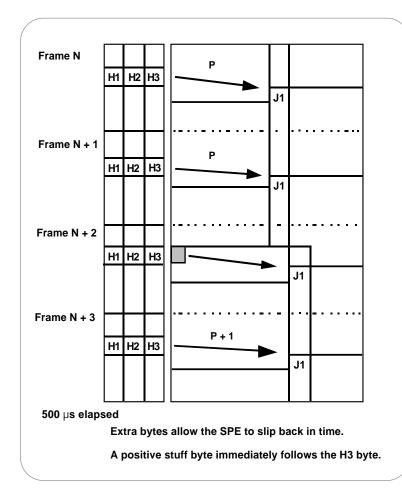
Figure 11. Payload pointer – positive justification.
