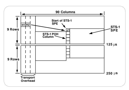
► Figure 10. Pointer – SPE position in the STS-1 frame.
