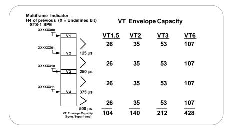
Figure 16. VT superframe and envelope capacity.
