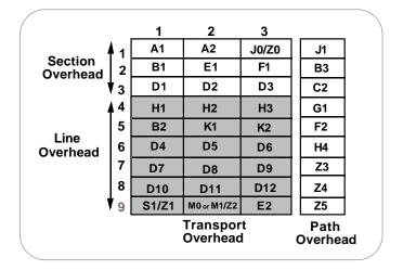
► Figure 8. Line Overhead — Rows 4 to 9 of Transport Overhead.
