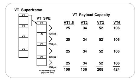
Figure 17. VT SPE and payload capacity.
