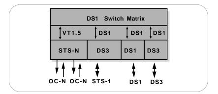
Figure 22. Wideband digital cross-connect.
