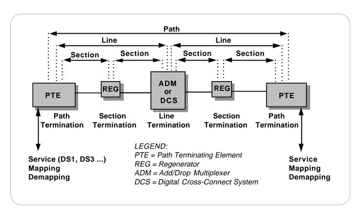
Figure 6. Overhead layers.
